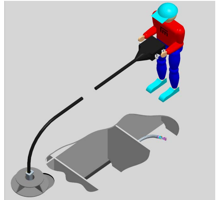
Inspection Probe Installed in Tank. Operated by person outside tank
