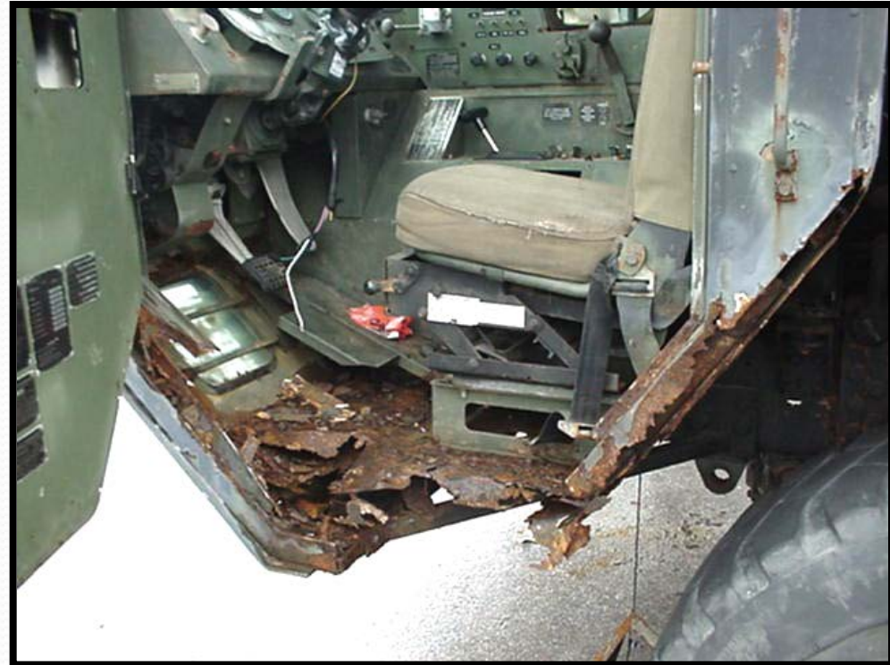
USMC Truck Ranked CC-4: “Item requires repair at the intermediate level before painting”
