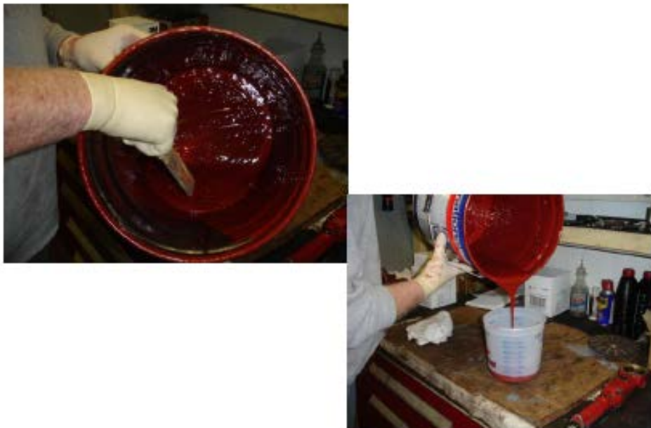
Mixing & Scraping Paint Interbond 998
