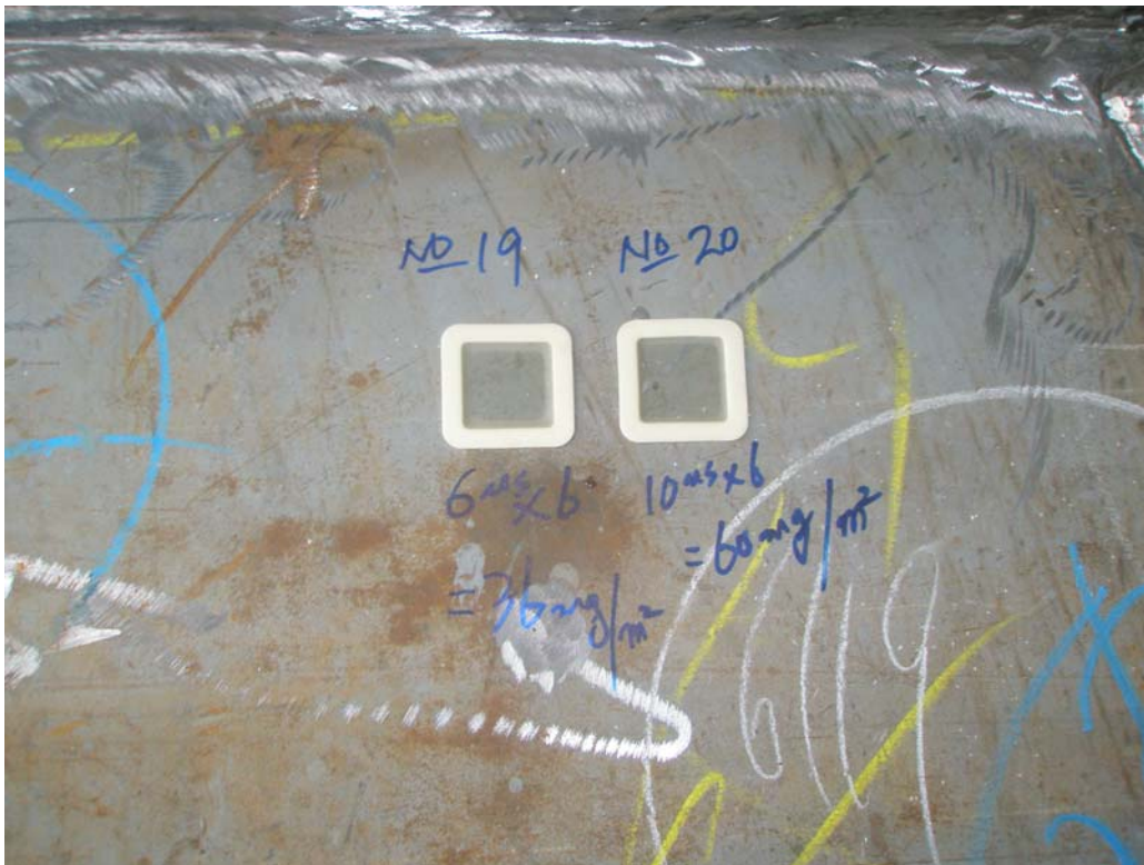
Block on an area with rust stain contamination over-head -Not expected to be contaminated by human traffic! Below, outer bilge area on the bottom plate.
