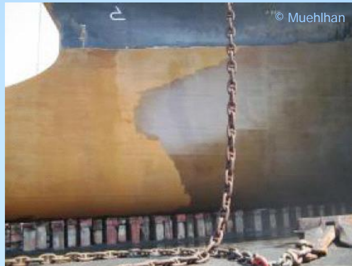
Wet blast cleaning
