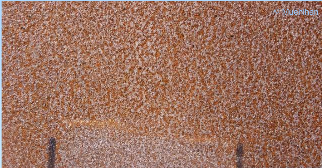
Tape-Test after WAB cleaning
