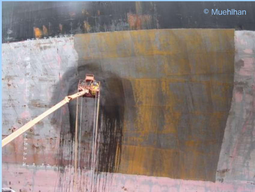
Wet blasting at high relative humidity (70%)
