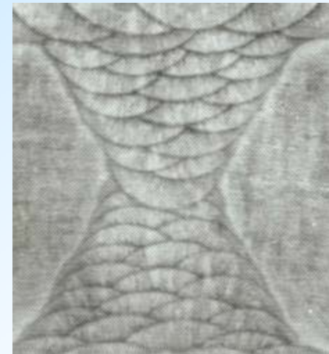
GTAW of 2-Inch Thick Titanium
