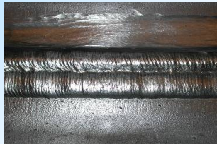
Ti-CP Weldment Produced with Double Pulse/Droplet Waveform
