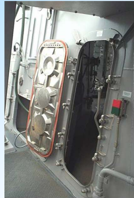
SPF/DB Ti Door Installed on DDG-51
