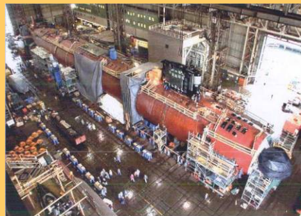
CCSM Off-Hull Test Pressure Hull Complete
