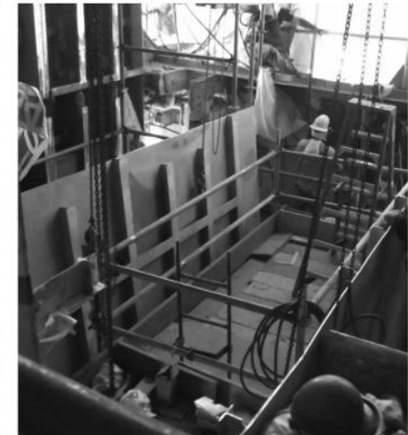
Structural Ship Alteration Expanded for the Gas Turbine Air Intake on Specific CG-47 Ships to Renew Adjacent Aluminum Alloy Plate
