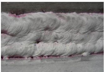
Weld Solidification Ripples Providing a Known Process Variable for PT Interpretation with Indication Relevancy
