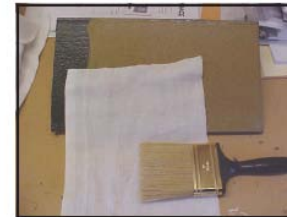
Photo 1 – Standard woven cotton cloth and 4-inch nylon bristle brush used for the brush-cloth wiping test.
