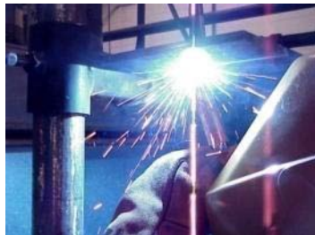
Gas Metal Arc Welding (GMAW)
