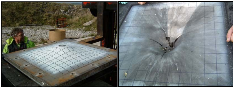
Mine blast test (800g C4 at 75mm standoff)
