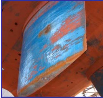
DDG-99 Cavitation Damage PSA Docking
