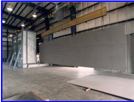
Fully automated Wheel-a-brator Up to 25, 10' x 40' steel plates per shift
