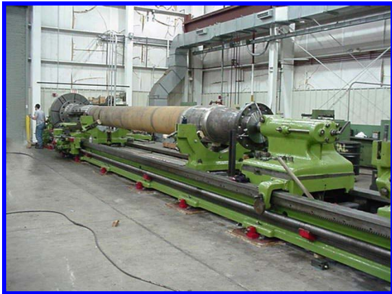
70' Lathe with 72" turn
