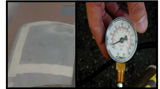
A ship radome section (left) is stripped at low pressure (right) using the CHP blasting process
