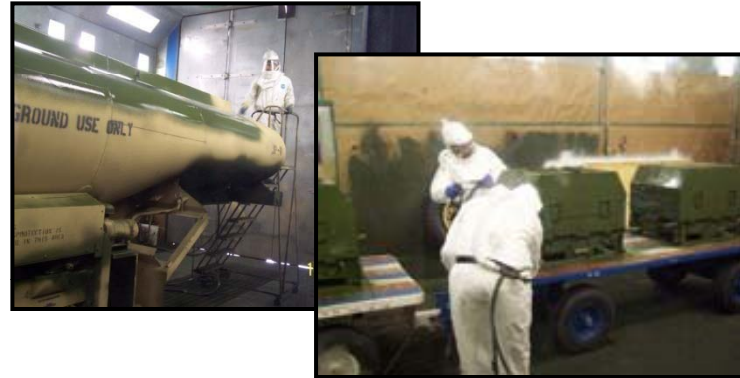
Water-Reducible CARC transitioned to Combat Equipment Group–Afloat, Goose Creek, SC, reducing hazardous air emissions and worker exposure
