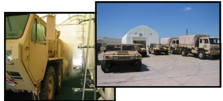
In preparation for overseas deployment, Ft. Hood vehicles are treated with a corrosion inhibitor, extending vehicle service life and increasing mission readiness
