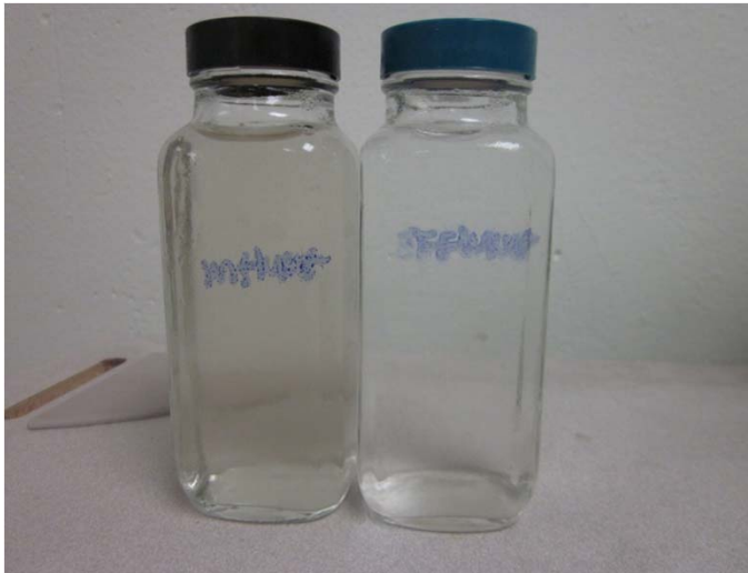
Fig. 1. Stormwater- before (Influent) and after treatment (Effluent).
